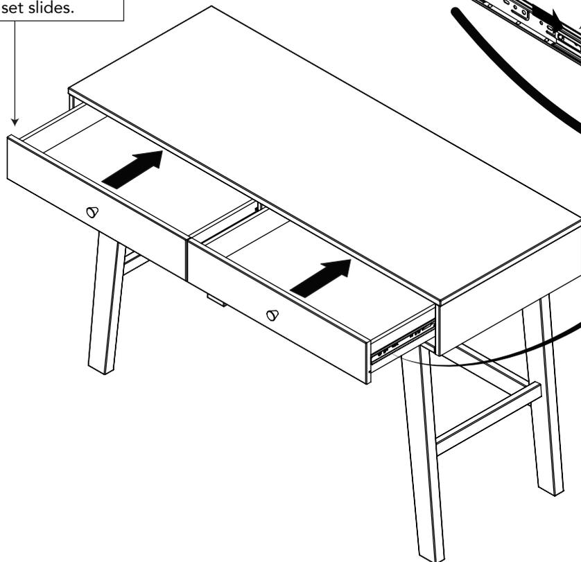
These slide sections mounted on desk must be fully extended for install.
